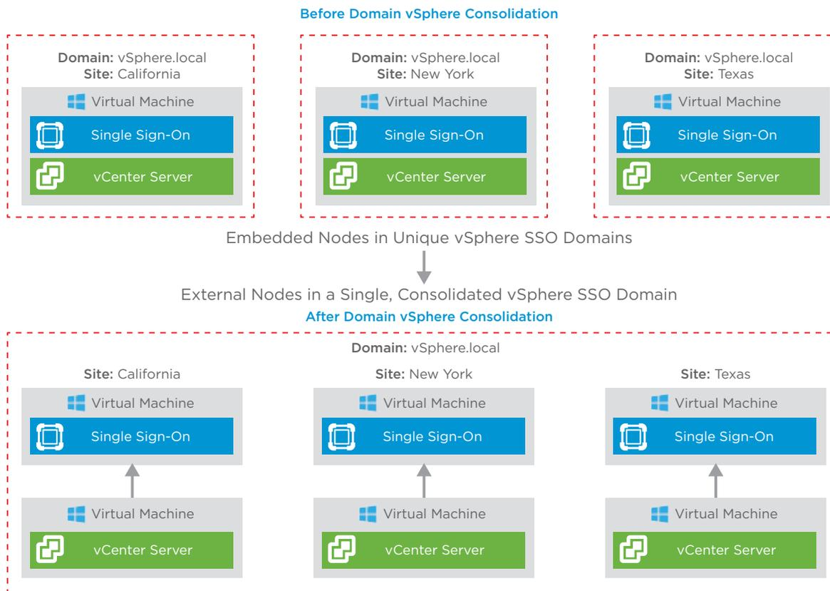
**Figure 1:** Performing vSphere SSO Domain Consolidation.
