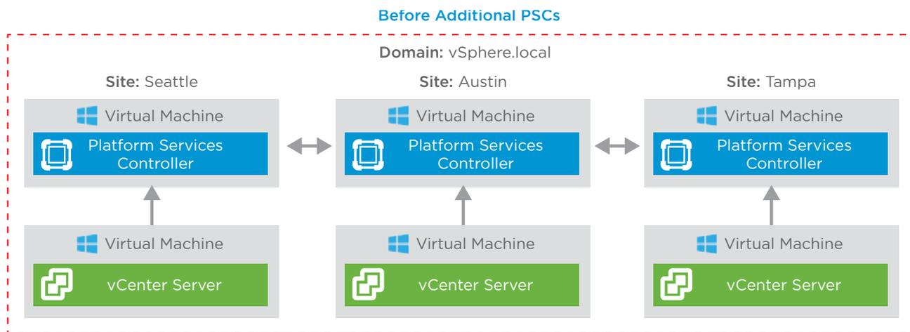
**Figure 3:** Environment Prior to vSphere Upgrade
