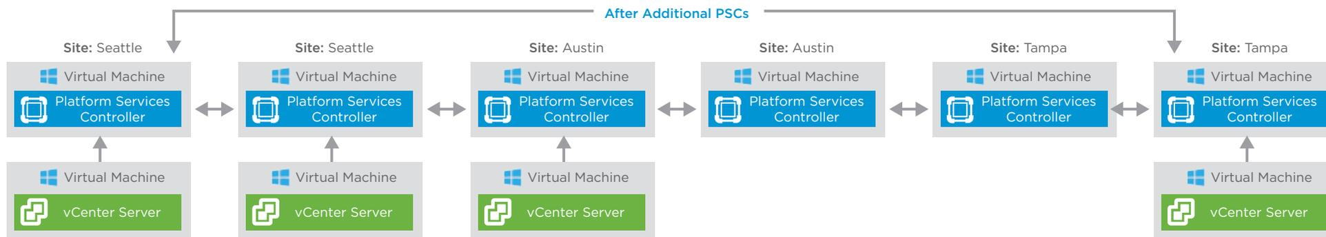
**Figure 5:** vSphere SSO Domain Built with a Ring Topology
